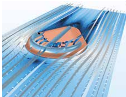
▼ Model of the CFD around a prehistoric animal. The optimal position of the feeding organ (sort of mouth) would be in the recirculation zone behind the arms of the anchor-shaped structure, where solid nutrients would settle on the surface of the animal. (Model reproduced from Darroch et al, https://royalsocietypublishing.org/doi/full/10.1098/rsbl.2017.0033 )
