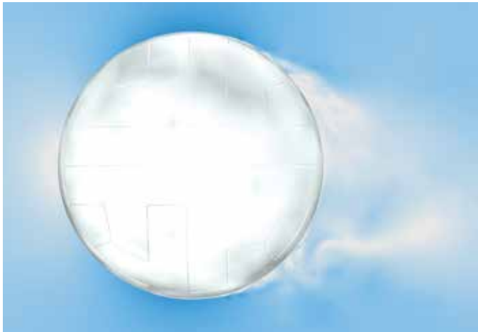
▼ Flow field around a football travelling at 20m/s (the speed of a cross that you can head). This looks like a relatively simple problem but it requires millions of degrees of freedom and advanced models, in this case large eddy simulations (LES), in order to obtain relatively accurate values of drag and lift. The solution shown in this figure takes days to compute on a desktop computer just to simulate half a second of flight
